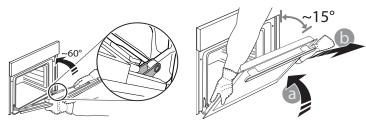
Refit the door by moving it towards the oven, aligning the hooks of the hinges with their seating and securing the upper part onto its seating.
