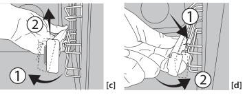
**REMOVING AND REFITTING THE SHELF GUIDES 1.** To remove the shelf guides, firmly grip the external part of the guide, and pull it towards you to extract the support and the two internal pins from the lodging.
